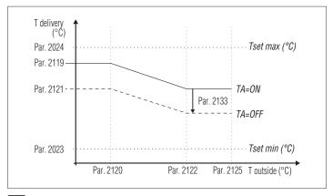
If the external probe (accessory) is not detected (not installed or damaged), the system makes a heat request at the maximum setpoint set on the climatic curve.
