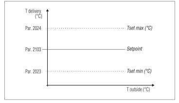
**Mode 1:** Operation with ambient thermostat (AT/OT) heat request and external probe (accessory)
