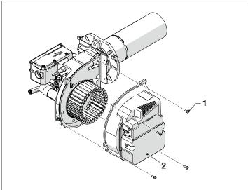
Reverse the above steps to reassemble. Take care to replace all burner parts in their original positions.
