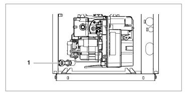
Open the shut-off devices of the hydraulic system and slowly load until the display shows the value, with cold water, of 1,5 bar
