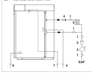
A Domestic hot water and central heating circuits must be completed with expansion vessels of adequate capacity and suitable, correctly-sized safety valves. The discharge of safety valves and appliances must be connected to a suitable collection and disposal system (see Catalogue for compatible accessories).
