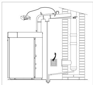
(\*) The sampling hole for flue gas analysis must be made on the straight section of the discharge duct, sufficiently far from curves and elbows. For the hole size and its correct positioning on the discharge duct (minimum or maximum distance from the equipment outlet to be observed), refer to the regulations in force.
