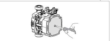
Check that the thermal unit has come to a complete stop by setting the main switch of the equipment and the main switch of the system to "off".
