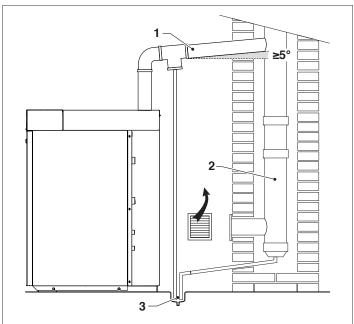
The condensate drain system (3) must conform to national and local legislation and standards.
