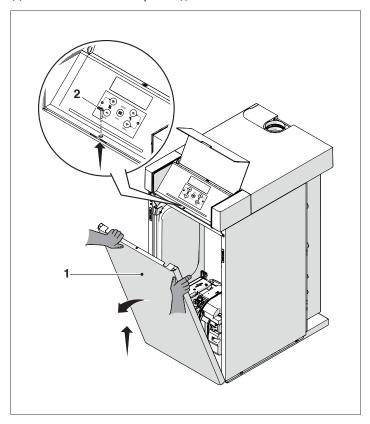
Locate the bag containing the documentation, extract the energy label and apply it to the boiler casing.
