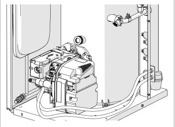
The light oil supply delivery pipe must be connected directly on the filter (1) (accessory), the return pipe to the preset union (2). Make sure that these connections are oil tight.
