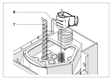
remove any displaced soot through the combustion chamber hole.
