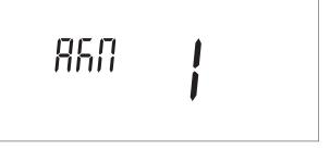
At first start-up and at every restoration of the power supply the venting function signalled by the message "Air" activates. The vent cycle lasts 14 minutes.
