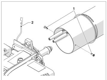
A With the blast tube removed, check its front edge to make sure that it is smooth, free from deposits, burns and dents.
