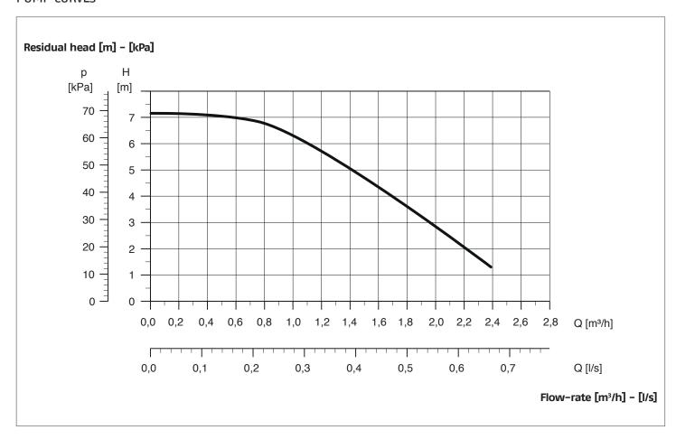
The curves refer to a density of 983.2 Kg/m³, a water temperature of +20°C and a kinematic viscosity of 0.474 mm²/s (0.474 cSt).
