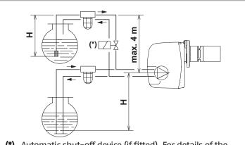
(\*) Automatic shut-off device (if fitted). For details of the electrical connections, see the "Automatic shut-off device (DAI)" section on page 26.
