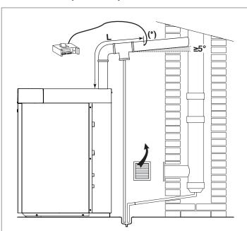
(\*) The sampling hole for flue gas analysis must be made on the straight section of the discharge duct, sufficiently far from curves and elbows. For the hole size and its correct positioning on the discharge duct (minimum or maximum distance from the equipment outlet to be observed), refer to the regulations in force.
