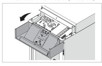
Lift the upper panel (4) and insert the external connection cables into the preset cable glands (5);
