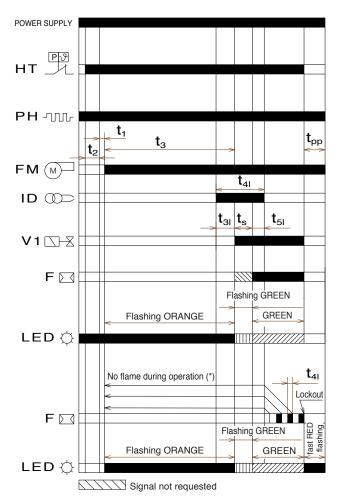
HT Heat request PH Pre-heater FM Fan motor
