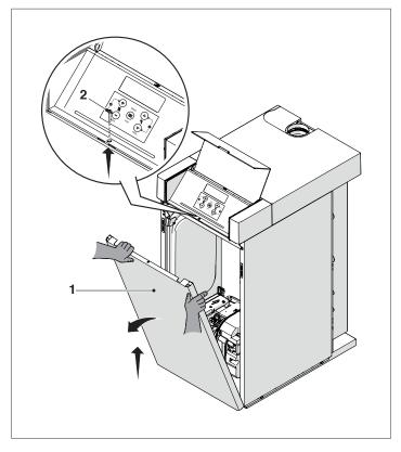
remove the fixing screw (3) from the top of the control panel;
