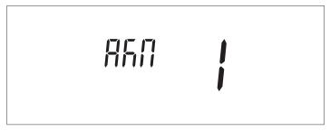
At first start-up and at every restoration of the power supply the venting function signalled by the message "Air" activates. The vent cycle lasts 14 minutes.
