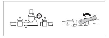
⚠ Drain the central heating circuit if there is any risk of freezing.
