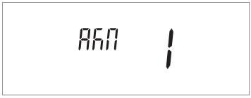
At first start-up and at every restoration of the power supply the venting function signalled by the message "Air" activates. The vent cycle lasts 14 minutes.
