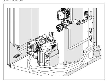
The light oil supply delivery pipe must be connected directly on the filter (1) (accessory), the return pipe to the preset union (2). Make sure that these connections are oil tight.
