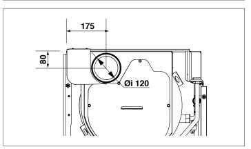
**INSIEME EVOe 32 V LN** boilers derive their comburent air from the room in which they are installed. Suitable air vents must therefore be provided in compliance with applicable laws and standards.
