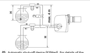
(\*) Automatic shut-off device (if fitted). For details of the electrical connections, see the "Automatic shut-off device (DAI)" section on page 25.
