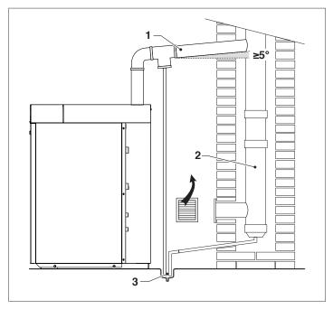
The condensate drain system (3) must conform to national and local legislation and standards.
