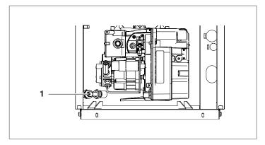
Open the shut-off devices of the hydraulic system and slowly load until the display shows the value, with cold water, of 1,5 bar
