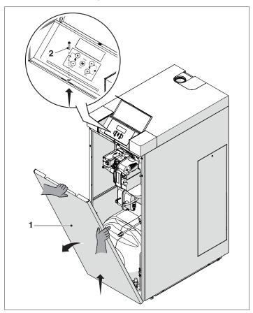
Locate the bag containing the documentation, extract the energy label and apply it to the boiler casing.
