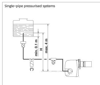
VIC: Fuel shut-off valve (where provided) For connecting the electricity, see paragraph "Fuel shut-off valve VIC (not supplied)".
