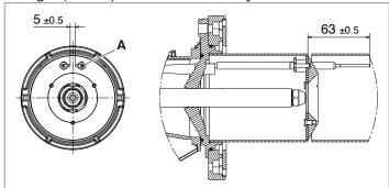
$\Delta$  It is essential to respect the dimensions in the figure. **REMOVING THE ELECTRODES**
