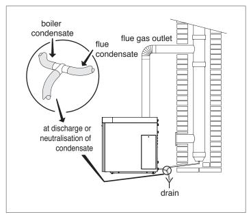
Any condensate neutralisation devices can be connected after the siphon. For the calculation of the duration of the neutralisation load, the amount of neutraliser consumption must be evaluated after one year of operation. The total duration of the load can be extrapolated from this information.
