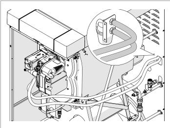
The connection to the light oil pump suction must be made directly on the filter (1) (accessory); the return pipe must be connected to the preset union (2).
