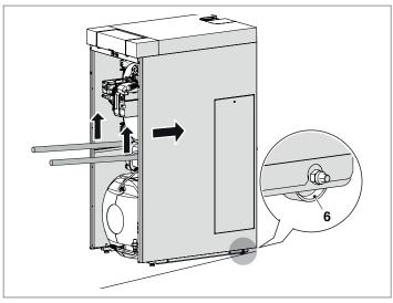
Level the thermal unit by acting on the 2 feet on the front side of the thermal unit.
