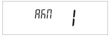
At first start-up and at every restoration of the power supply the venting function signalled by the message "Air" activates. The vent cycle lasts 14 minutes.
