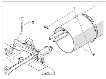
With the blast tube removed, check its front edge to make sure that it is smooth, free from deposits, burns and dents. Reverse the above steps to reassemble.
