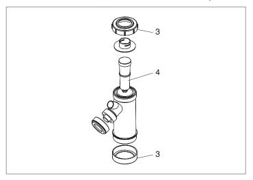
Once the maintenance operations are complete, refit the components working in the opposite direction of what was described.
