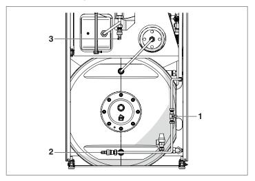
Open the system load valve (1) and slowly load until the display reaches the water pressure value (cold water) of 1.5 bar
