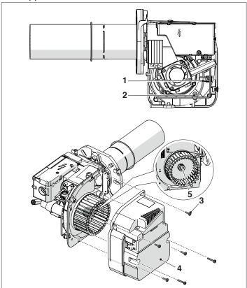
Mhen reassembling the fan, it is important to put it back in the correct position (B) and tighten the screw (5).
