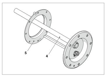
On completion of cleaning, refit all removed parts in the reverse order, taking care to ensure the efficiency of the seals.
