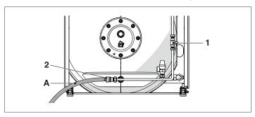
**NOTE** Open a hot water tap to facilitate emptying the storage cylinder.
