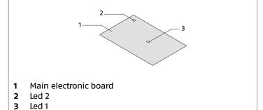
The unit operation is signalled with LED 2.
