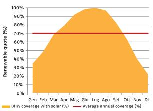
Simulation carried out in Rome, with panels exposed to the south and ACS requirements estimated at 50 liters per day per person. The simulation does not replace the technical / executive project of the solar system carried out by a Thermotechnical Designer.
