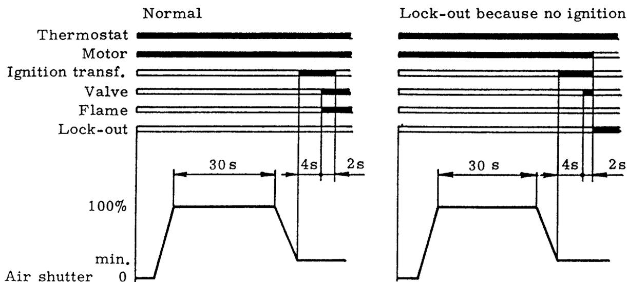
If during operation the flame shut off, lock-out occurs within 1 sec.
