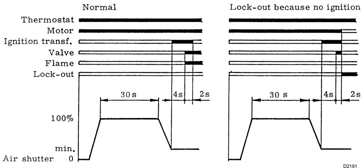
If during operation the flame shuts off, lock-out occurs within 1 sec.
