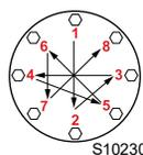
Tighten the nuts gradually (first to 30%, then to 60% up to 100%) according to the cross pattern shown in the figure.
