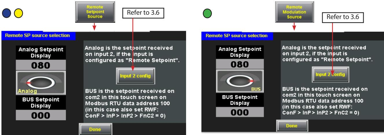
A remote setpoint can be sent to the burner via 0-20ma/4-20ma/0-10vd hardwired or bus signal.
