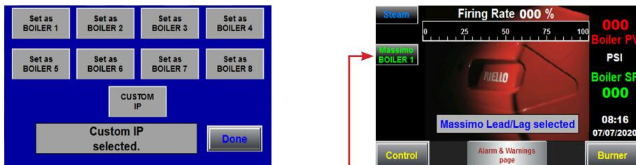
After selecting boiler number, recycle power on the burner. THIS IS VERY IMPORTANT!
