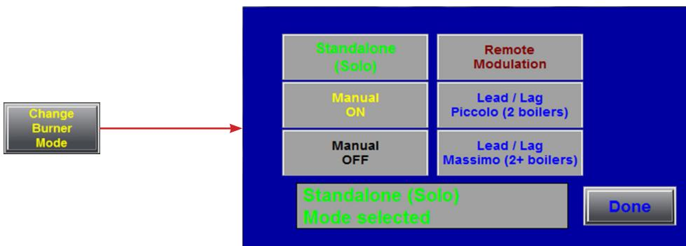
**Standalone (Solo):** The burner will use local or remote setpoint to modulate and maintain the process value (PV), without any external intervention. When the selected media is steam and hot standby is active, sending a setpoint of 0 PSI will shut down the burner, however the boiler will be kept warm within the limits of the hot standby routine.
