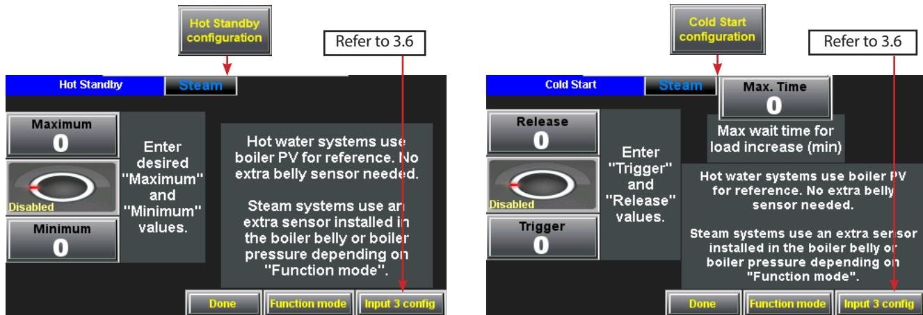
Boiler "Hot Standby" will be activated if the water temperature drops below "Minimum". The burner will start and enter Hot Standby" even if there is no call for heat.
