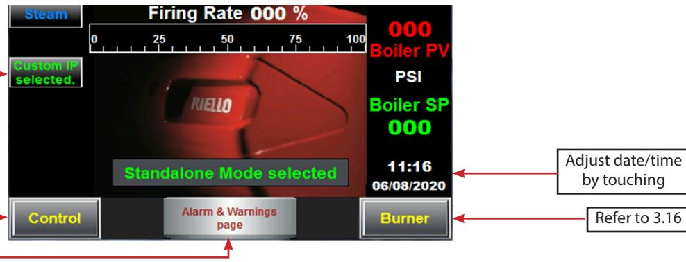
The burner screen gives an over-all general picture of the what is happening with the burner.
