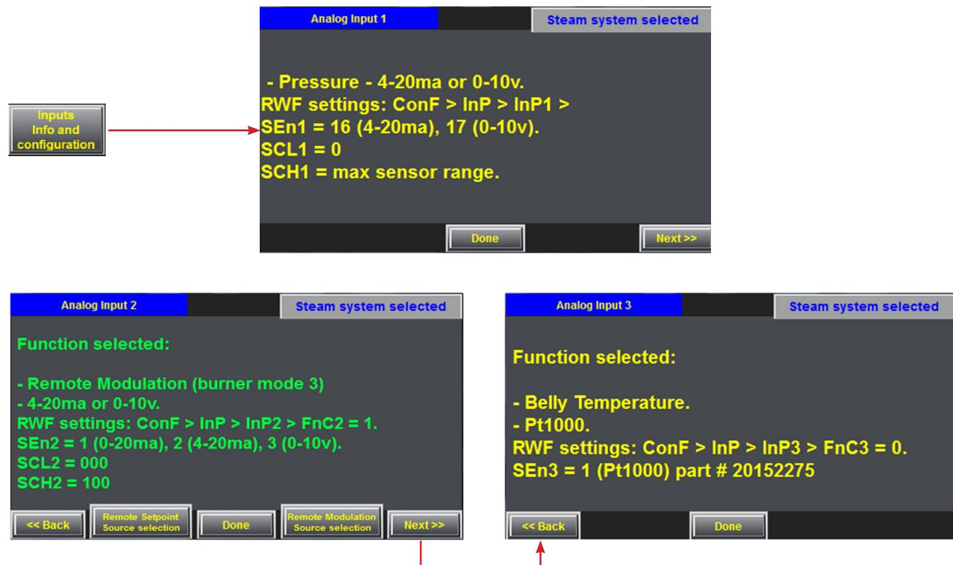
When using Burner with LMV3 and RWF55 Help screens are available to assist the technician properly set up the RWF55 to work with the touchscreen.
