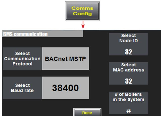
If a Riello gateway is connected to the Riello burner, it is configured in "BMS communication". The S3 dip switch has to be in the off position
