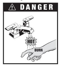
NOTE: (for heating only model): When this boiler is supplying general purpose hot water for use by individuals, a thermostatically controlled mixing valve for reducing point of use water temperature is recommended to reduce the risk of scald injury. Contact a qualified plumber or the local plumbing authority for further information.
