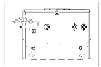
Before filling or draining the system, switch the system's master switch to the OFF position and the boiler's master switch to (0).
