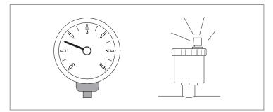
NOTE: The system must be filled up slowly the first time; once it is filled and the air is expelled it should never need to be topped up again.
