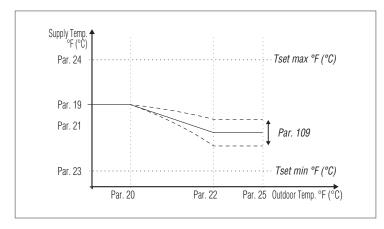
The demand is activated when the room/heat demand thermostat's contact is closed provided that outdoor temperature does not exceed the value set by the parameter 25.
