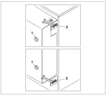
With the door open, remove the hinge assembly 'B' (bushing, bolt, and washer) opposite the pivot side of the door.
