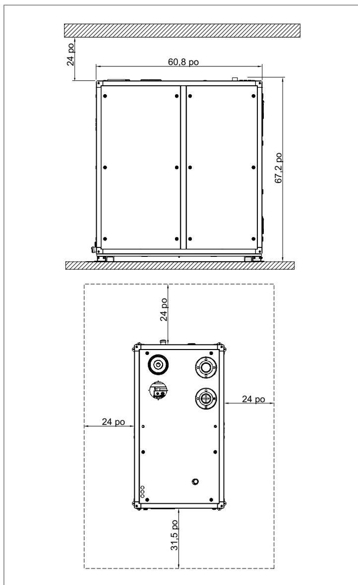
Fig. 3 Array AR 1000, AR 1500 Clearances
