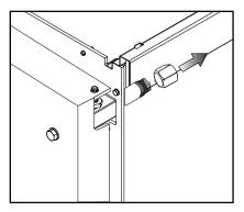
Open the door and use a hacksaw or file to remove the cutout from the front head on the opposite side to the door hinges. Reclose the door and secure it with the bolts (2). Remove the plug (1), taking care not to lose the spring from inside the threaded tube.
