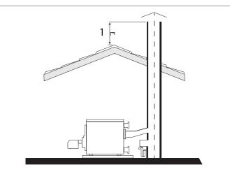
Flue must be isolated. Isolation ratio is:  $\Delta t < 1^{\circ}C/m$  Minimun flue highth must be 6 m.
