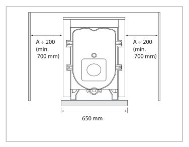
The recommended height for the boiler room is at least 2,200 mm, leave the minimum space free on the sides and in front of the boiler as shown in the drawing.
