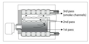
The 3-passageway system brings about the forced circulation of the combustion gas inside the boiler three times before it comes out of the discharge pipe. In this way, all the useful thermal energy is transferred to the water inside the elements. The optimised combustion chamber and the excellent thermal insulation provide maximum energy efficiency.
