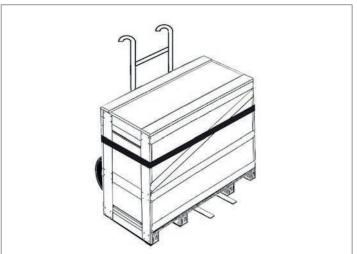
When the boiler is being stored or transported ensure at least the normal storage conditions (non-aggressive environment, air humidity less than 75%, temperature between 5° and 55° C, low dust levels and the prevention of damage due to biological factors).
