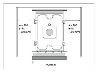
The recommended height for the boiler room is at least 2,200 mm, leave the minimum space free on the sides and in front of the boiler as shown in the drawing. Provide a base with a minimum height of 200 mm above the floor for the installation of the burner of the boiler.
