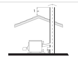
Flue must be isolated. Isolation ratio is:  $\Delta t < 1^{\circ}C/m$  Minimun flue highth must be 6 m.
