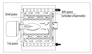
The 3-passage system brings about the forced circulation of the combustion gas inside the boiler three times before it comes out of the discharge pipe. In this way, all the useful thermal energy is transferred to the water inside the elements. The optimised combustion chamber and the excellent thermal insulation provide maximum energy efficiency.
