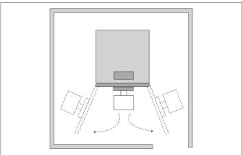
Provide enough space for the tools to be used in the boiler room.
