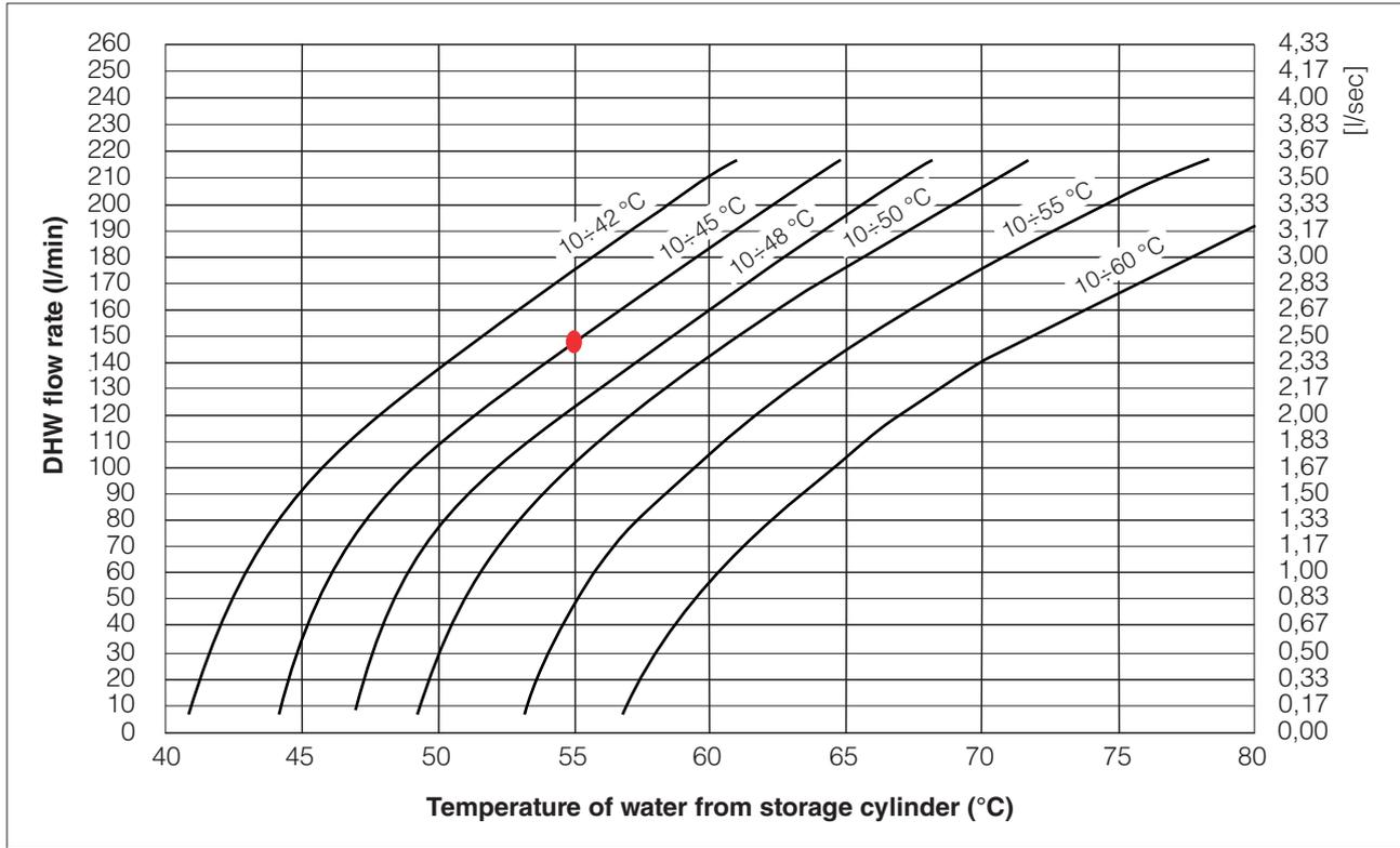
**NB:** The proper working of the module is assured if the supply temperature of the primary circuit is at least 3°C greater than the DHW temperature set.
