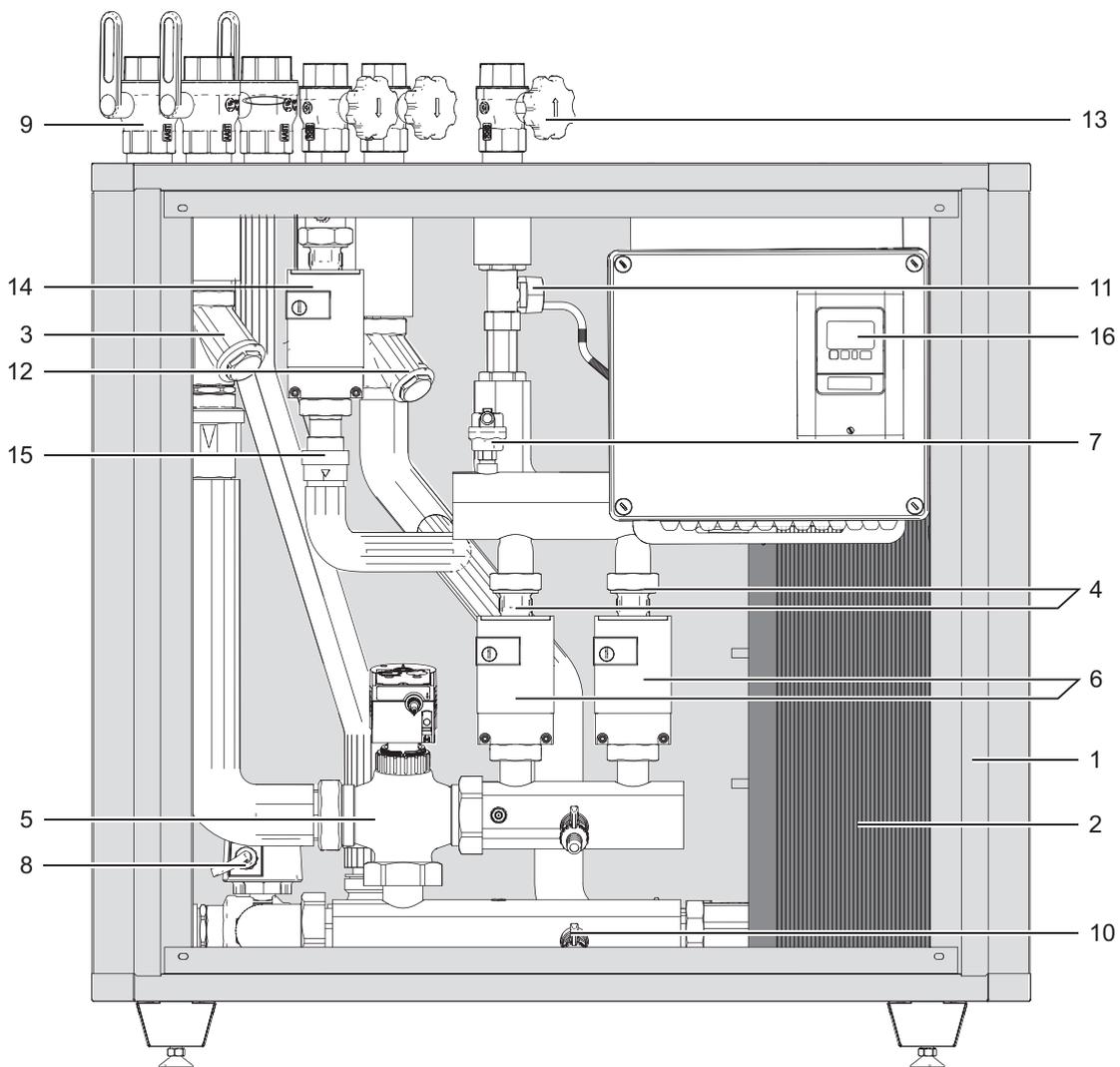
1 Cabinet in painted steel sheet, ventilation slots for internal electronic components, and inspection access on all four sides
