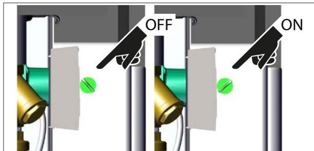
**The recirculation kit, not as the primary circuit, requires a manual venting operation, by acting on the special valve located above the circulator. The same is connected to a drainage tube. It is advisable to carry out the bleeding operations by slightly opening the valve and using a suitable container to avoid splashing water against the electrical parts of the BIG T-FAST.**
