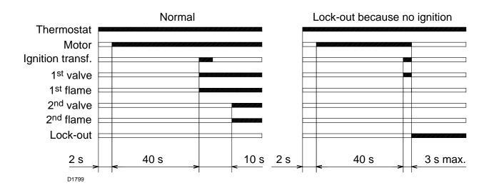
If during operation the flame shuts off, lock-out occurs within 1 sec.
