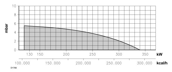
Min. output at 1st stage: 80 kW - 69.000 kcal/h.
