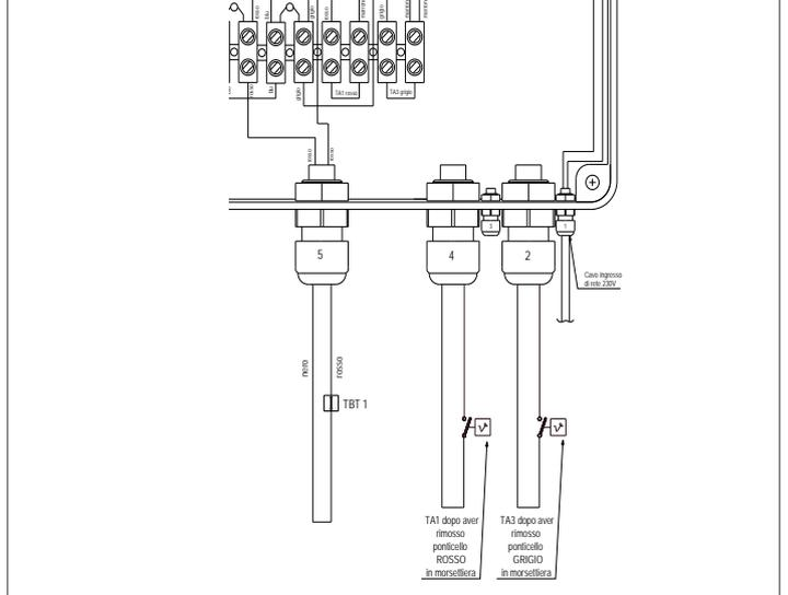
**!** The ambient thermostats (TA) and/or chrono-thermostats (CT) of the low and high temperature systems must be connected directly to the **BAG<sup>3</sup>** using a cable with a minimum section of 1 mm<sup>2</sup>.
