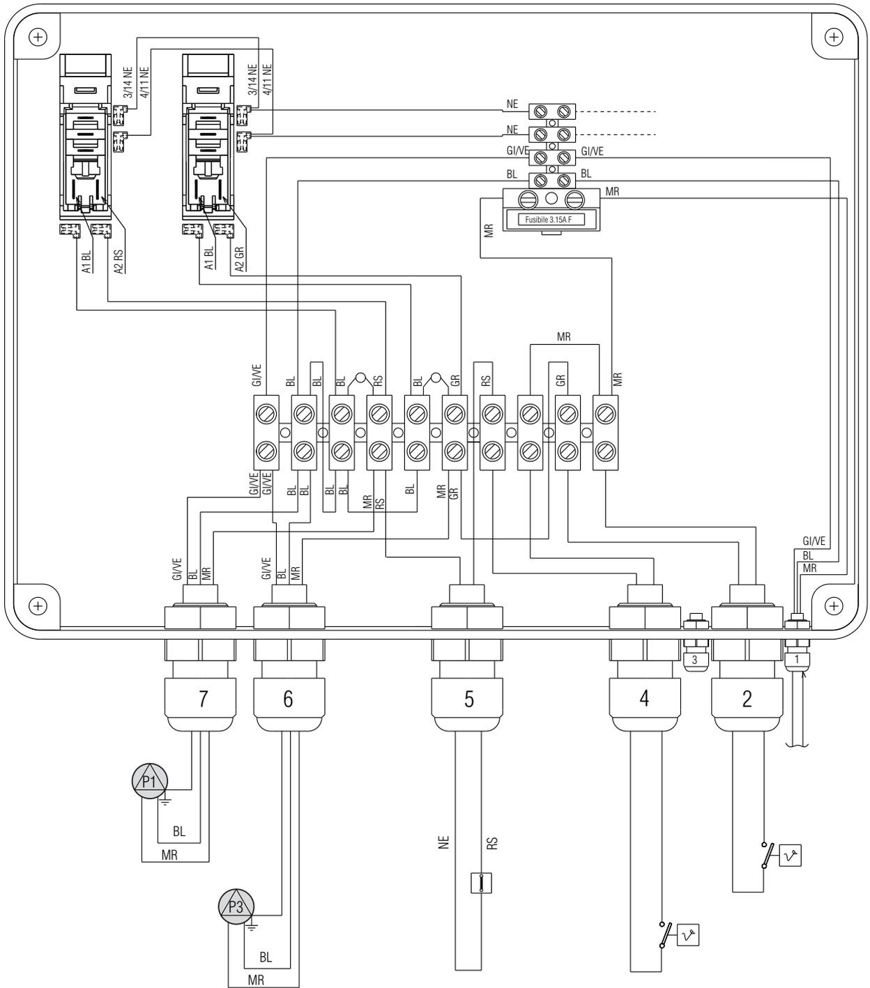
**!** If the wiring or the board are replaced, observe and respect all the connections of the cables according to the numbered sequence shown in the figure.
