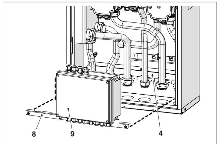
**!** The hydraulic module is supplied already wired to the drivers of the module itself. For other connections, please refer to the wiring diagrams in this document (see "1.9 Wiring diagram" page 21).
