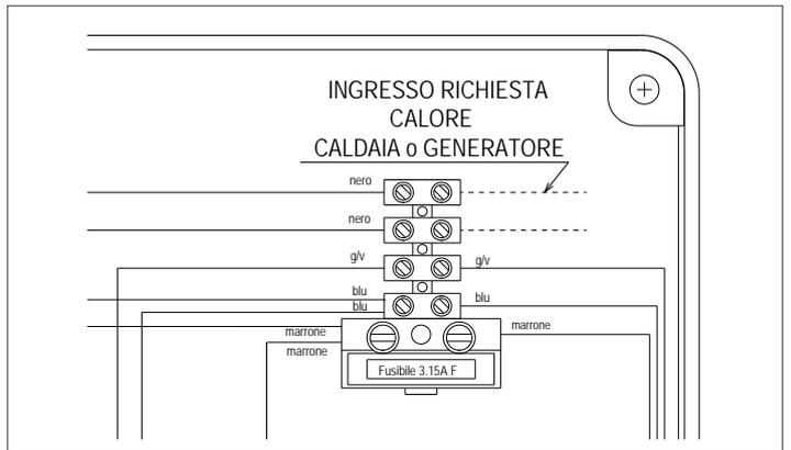
**!** Connect the mammut (B-B) of the **BAG<sup>3</sup>** to the mammut (TA) of the boiler using a cable with a minimum section of 2x0.5 mm<sup>2</sup> (please refer to the wiring diagram in the instruction booklet for the installer of the specific boiler).
