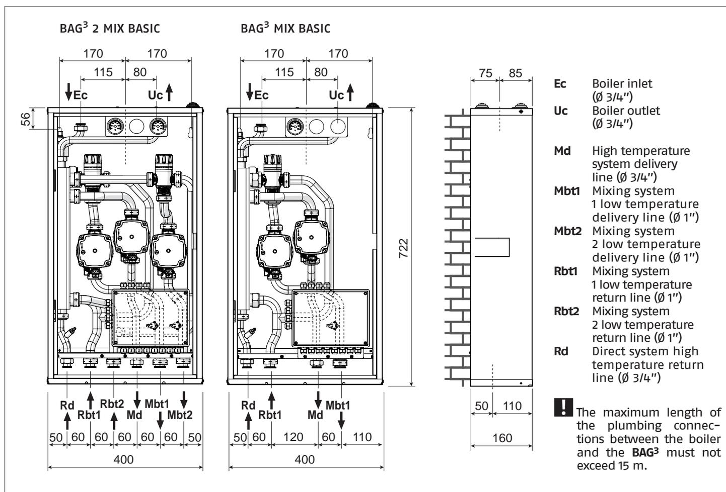
Before any of the connections are made, all the piping must be thoroughly flushed to remove any residue which could compromise the proper functioning of the BAG<sup>3</sup>.
