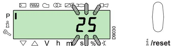
To return to the list of parameters, press the keys "+" and "-" (ESC) simultaneously.
