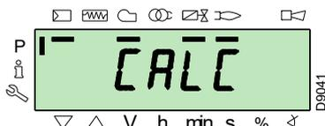
The flame control will automatically calculate the points from "P8" to "P2", distributing them in a straight line. These are theoretical and must be checked.
